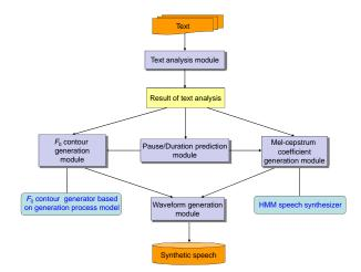
*Figure 1:* Total configuration of developed speech synthesizer.
