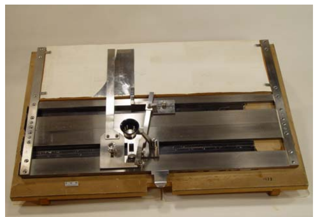
Figure 6: Improved version of the pitch contour measuring apparatus. Original device from the Hamburg Phonetic Institute, now in the Dresden collection.
