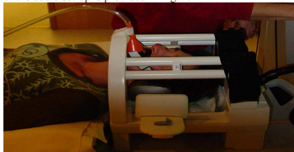
Figure 2: Experimental set-up designed to record subjects’ verbal production during an fMRI session.
