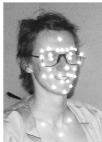
Figure 2: Test subject with the IR-reflecting markers glued to the face.
