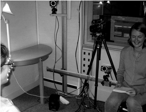
Figure 1: Data collection setup with video and IR-cameras, microphone and a screen for prompts.
